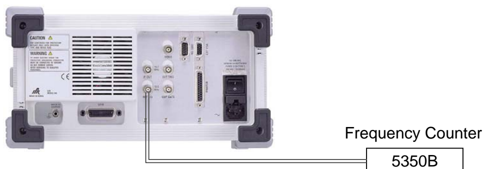
Figure 6-1. Reference Oscillator Frequency Stability Test
